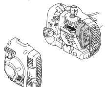
In countries that have a warm and dry climate there is a significant risk of fire. We therefore fit certain mufflers with a spark arrestor screen. Check whether the muffler on your machine is fitted with this kind of screen.
