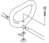
• Fit the bolt, securing plate and wing nut as shown in the diagram. Tighten the wing nut.
